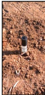
Figure 11. Fully Installed Access Tube.
